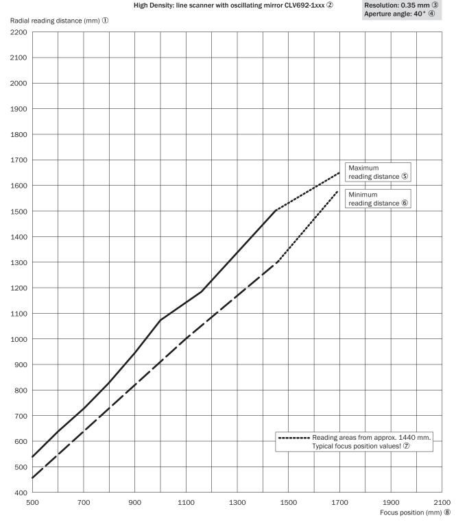
Figure 128: CLV692-1xxx (High Density): min. and max. radial reading distance depending on the focus position at a resolution of 0.35 mm and aperture angle of  $\alpha$  = 40 °
