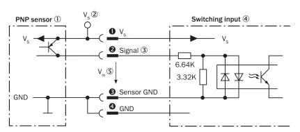
Figure 61: Wiring of a switching input with external PNP sensor
