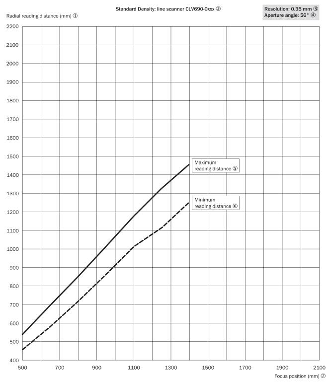
Figure 103: CLV690-0xxx (Standard Density): min. and max. radial reading distance depending on the focus position at a resolution of 0.35 mm and aperture angle of  $\alpha = 56^{\circ}$
