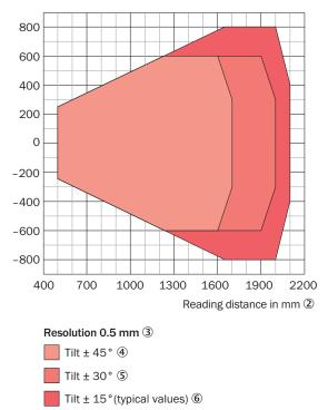
Figure 118: CLV691-1xxx (Low Density): reading field height depending on the reading distance and tilt at a resolution of 0.5 mm
