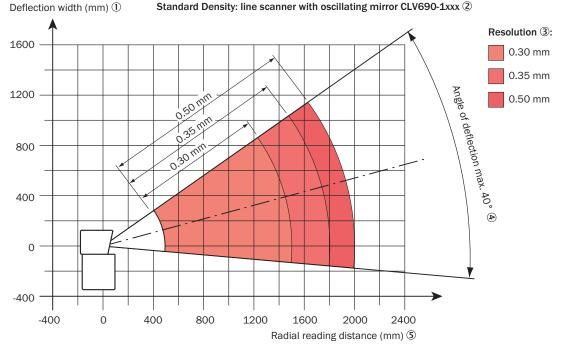
Standard Density: line scanner with oscillating mirror CLV690-1xxx ②
