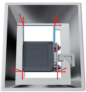
Figure 19: Mounting with mounting holder - taking the working distance into consideration
