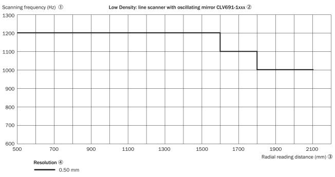
Figure 119: CLV691-1xxx (Low Density): characteristic curve field scanning frequency depending on the radial reading distance and resolution
