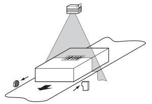
Figure 100: Cleaning the external optical sensors (read pulse encoder)
