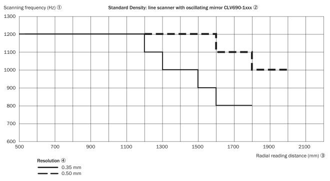
Figure 112: CLV690-1xxx (Standard Density): characteristic curve field scanning frequency depending on the radial reading distance and resolution
