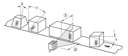
Figure 14: Line scanner: Read angle occurring between scanning line and bar code
