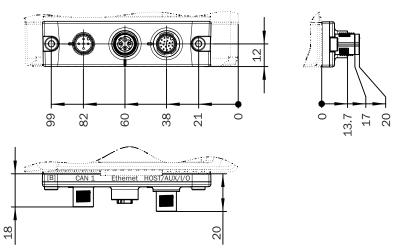
Figure 36: Dimensions of cloning plug B (M12), all dimensions in mm
