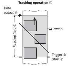
Figure 11: Tracking operating mode of the device in stand-alone operation
