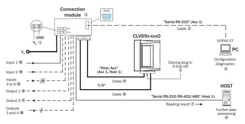
Figure 6: Facilities for connecting for devices without/with integrated heating to connection module CDM490-0001 when replacing a predecessor CLV49x
