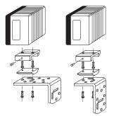
Figure 12: Example of mounting a CLV69x with a quick clamping device and a mounting bracket
