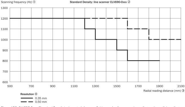
Figure 106: CLV690-0xxx (Standard Density): characteristic curve field scanning frequency depending on the radial reading distance and resolution
