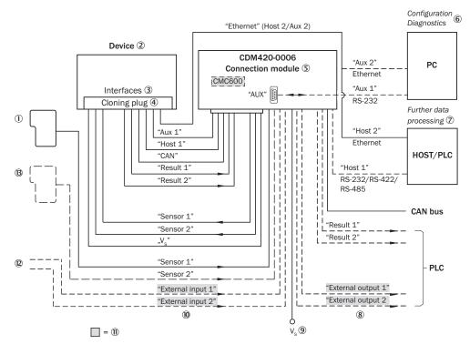
Figure 58: Connection of the device to the CDM420-0006 connection module
