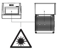
Figure 1: Laser output aperture in the different designs
