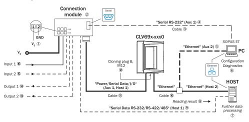
Figure 5: Facilities for connecting for devices without/with heating to connection module CDB650-204 or CDM420-0006
