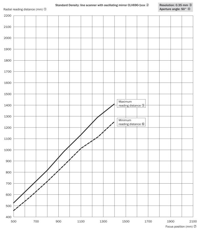
Figure 109: CLV690-1xxx (Standard Density): min. and max. radial reading distance depending on the focus position at a resolution of 0.35 mm and aperture angle of  $\alpha = 50^{\circ}$
