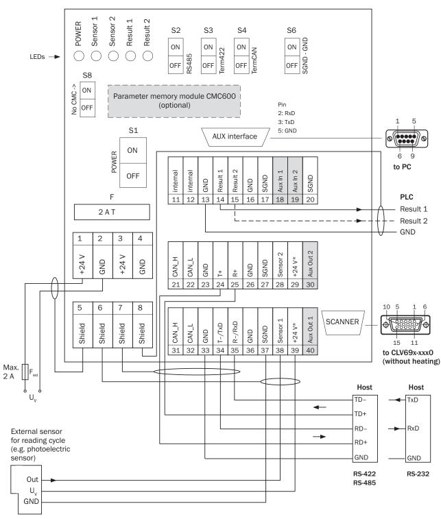
$U_v$  = DC 18 V ... 30 V for CLV69x-xxx0 (without heating) at terminal +24 V = +24 V\* after switch S1, protected by internal fuse F
