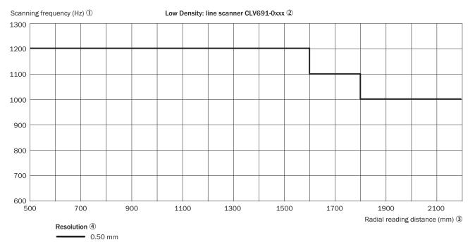
Figure 117: CLV691-0xxx (Low Density): characteristic curve field scanning frequency depending on the radial reading distance and resolution
