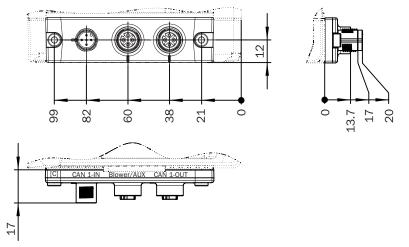
Figure 41: Dimensions of cloning plug C (M12), all dimensions in mm
