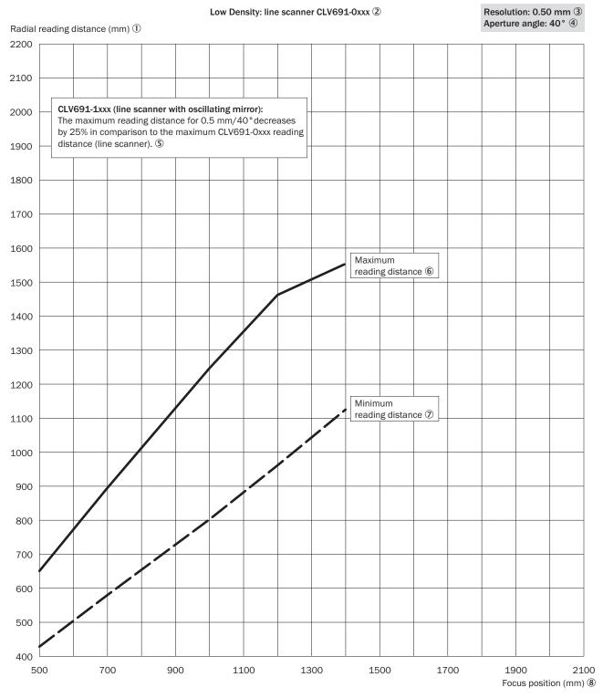
Figure 115: CLV691-0xxx (Low Density): min. and max. radial reading distance depending on the focus position at a resolution of 0.5 mm and aperture angle of  $\alpha$  = 40 °
