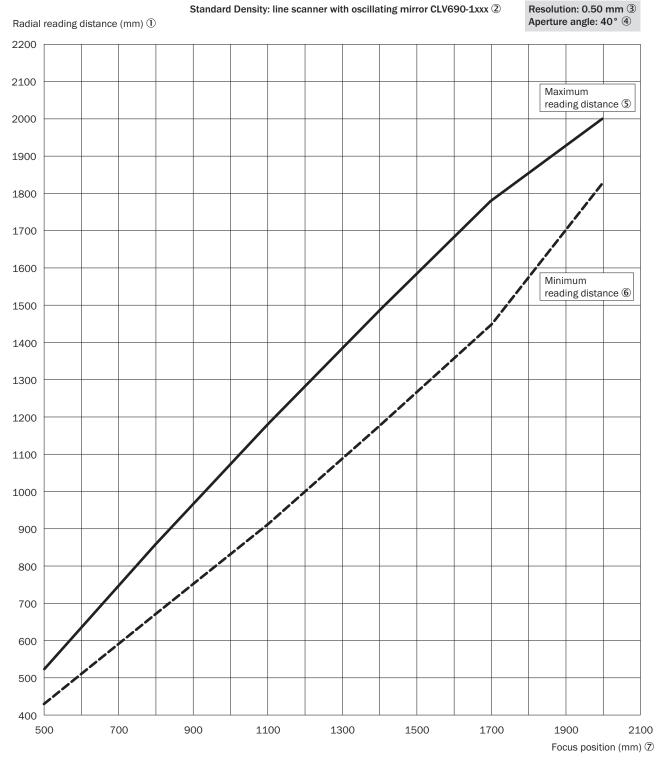
Figure 110: CLV690-1xxx (Standard Density): min. and max. radial reading distance depending on the focus position at a resolution of 0.50 mm and aperture angle of  $\alpha = 40^{\circ}$
