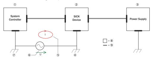
Figure 24: Example: Occurrence of equipotential bonding currents in the system configuration
