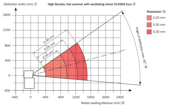
Figure 131: CLV692-1xxx (High Density): deflection width depending on the radial reading distance, angle of deflection and resolution
