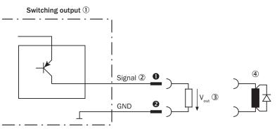
Figure 62: Wiring of a switching output
