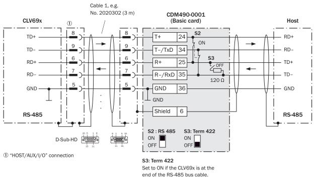
Figure 93: Wire serial host interface RS-485
