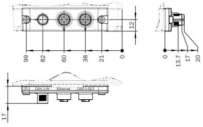
Figure 51: Dimensions of cloning plug E (M12), all dimensions in mm
