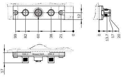
Figure 46: Dimensions of cloning plug D (M12), all dimensions in mm
