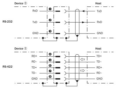
Figure 60: Internal circuitry for RS-232 and RS-485 data interfaces
