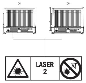
Figure 2: Example of a laser warning symbol on the device
