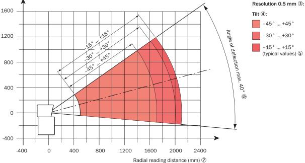
Figure 120: CLV691-1xxx (Low Density): deflection width depending on the reading distance, angle of deflection and tilt at a resolution of 0.5 mm
