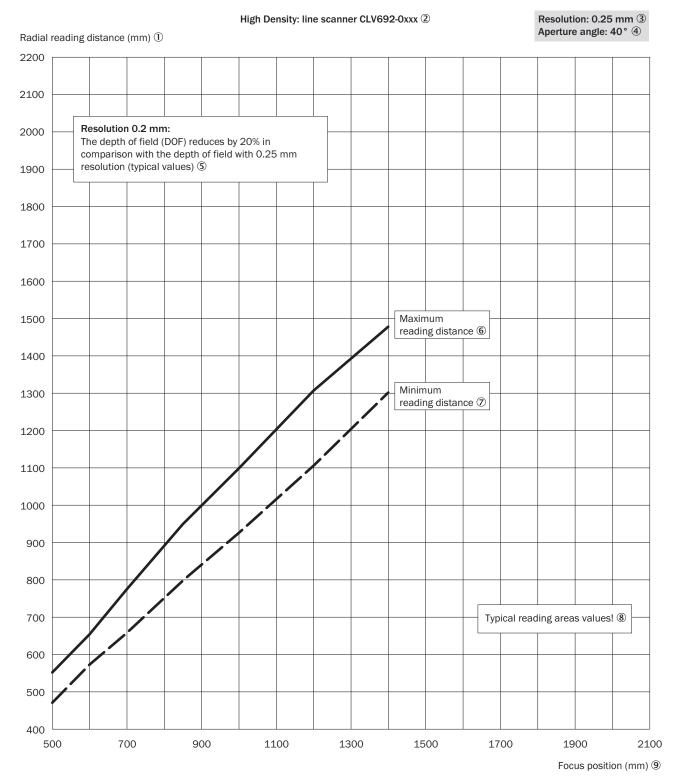
Figure 122: CLV692-0xxx (High Density): min. and max. radial reading distance depending on the focus position at a resolution of 0.25 mm and aperture angle of  $\alpha$  = 40 °
