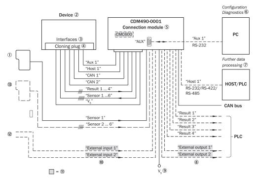
Figure 59: Connection of the device to the CDM490-0001 connection module
