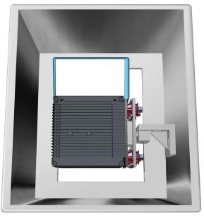
Figure 22: Mounting with mounting holder, oscillating mirror scanner, horizontal reading line
