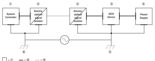
Figure 25: Example: Prevention of equipotential bonding currents in the system configuration by the use of electro-optical signal isolators
