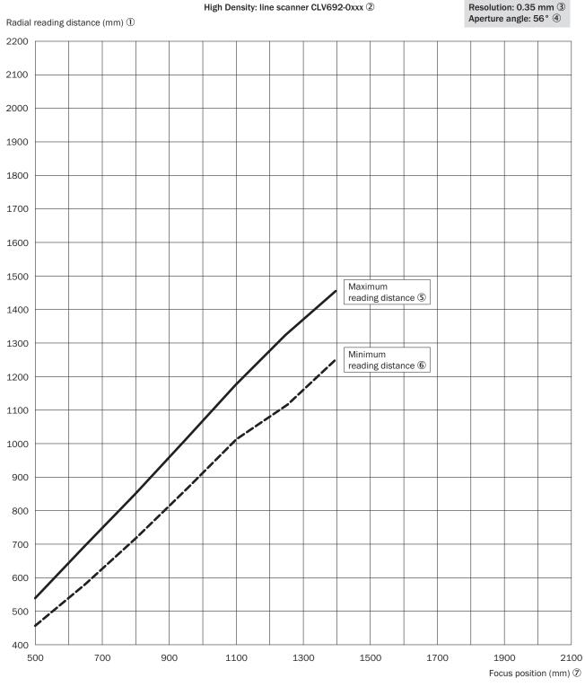
Figure 124: CLV692-0xxx (High Density): min. and max. radial reading distance depending on the focus position at a resolution of 0.35 mm and aperture angle of  $\alpha$  = 56 °
