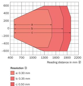
Figure 107: CLV690-1xxx (Standard Density): reading field height depending on the reading distance and resolution
