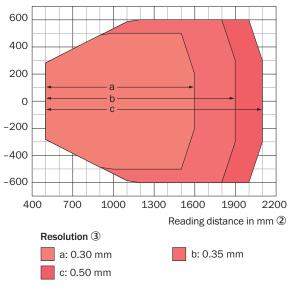
Figure 101: CLV690-0xxx (Standard Density): reading field height depending on the reading distance and resolution
