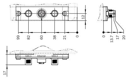
Figure 56: Dimensions of cloning plug F (M12), all dimensions in mm
