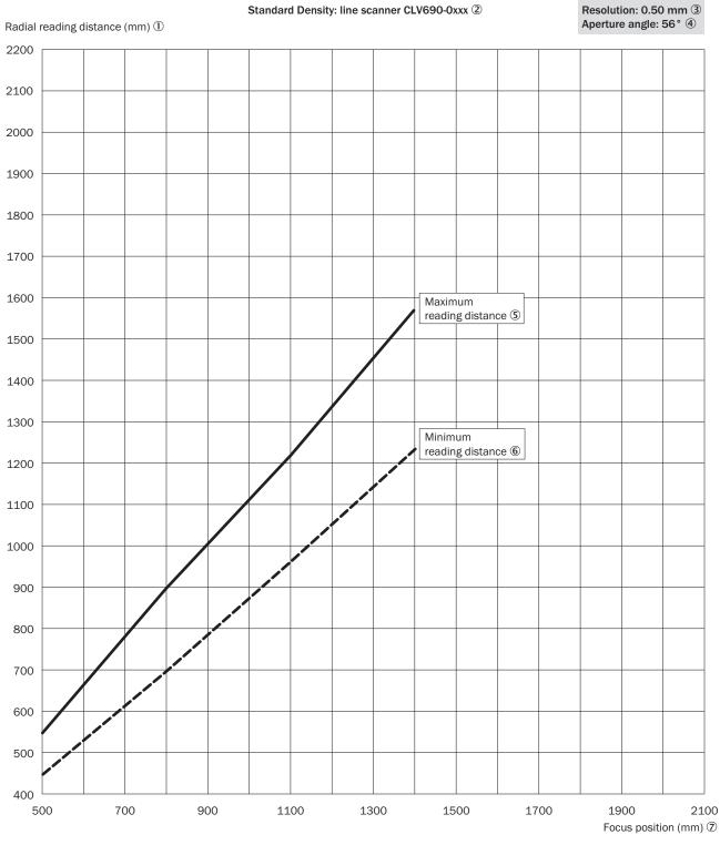
Figure 105: CLV690-0xxx (Standard Density): min. and max. radial reading distance depending on the focus position at a resolution of 0.50 mm and aperture angle of  $\alpha$  = 56 °
