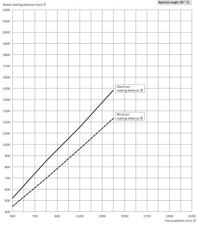
Standard Density: line scanner with oscillating mirror CLV690-1xxx 2
