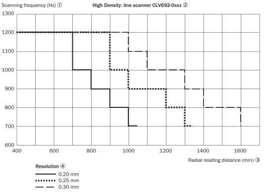
Figure 125: CLV692-0xxx (High Density): characteristic curve field scanning frequency depending on the radial reading distance and resolution
