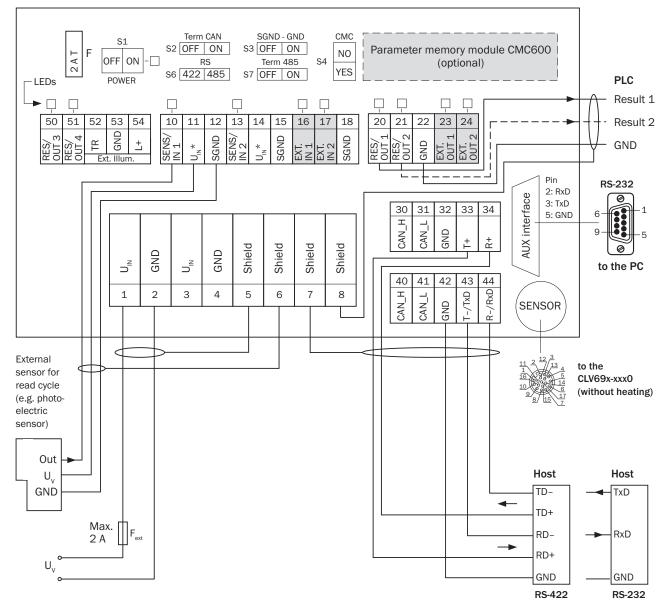
$\rm U_v$  = DC 18 V ... 30 V for CLV69x-xxx0 (without heating) at terminal  $\rm U_{_{\rm IN}}$  =  $\rm U_{_{\rm IN}}^*$  after switch S1, protected with internal fuse F
