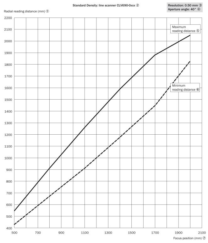
Figure 104: CLV690-0xxx (Standard Density): min. and max. radial reading distance depending on the focus position at a resolution of 0.50 mm and aperture angle of  $\alpha = 40^{\circ}$
