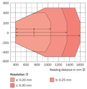
Figure 121: CLV692-0xxx (High Density): reading field height depending on the reading distance and resolution
