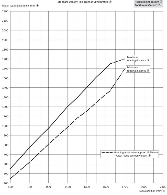
Figure 102: CLV690-0xxx (Standard Density): min. and max. radial reading distance depending on the focus position at a resolution of 0.35 mm and aperture angle of  $\alpha = 40^{\circ}$
