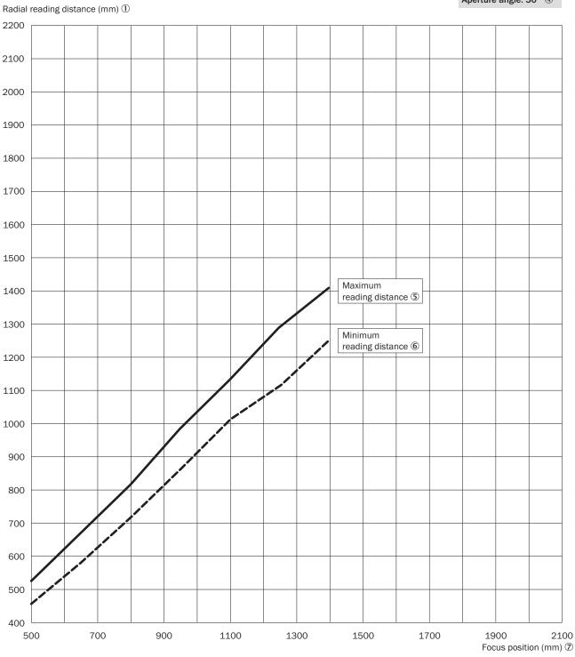
High Density: line scanner with oscillating mirror CLV692-1xxx 2
