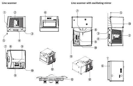
Figure 4: Line scanner and line scanner with oscillating mirror
