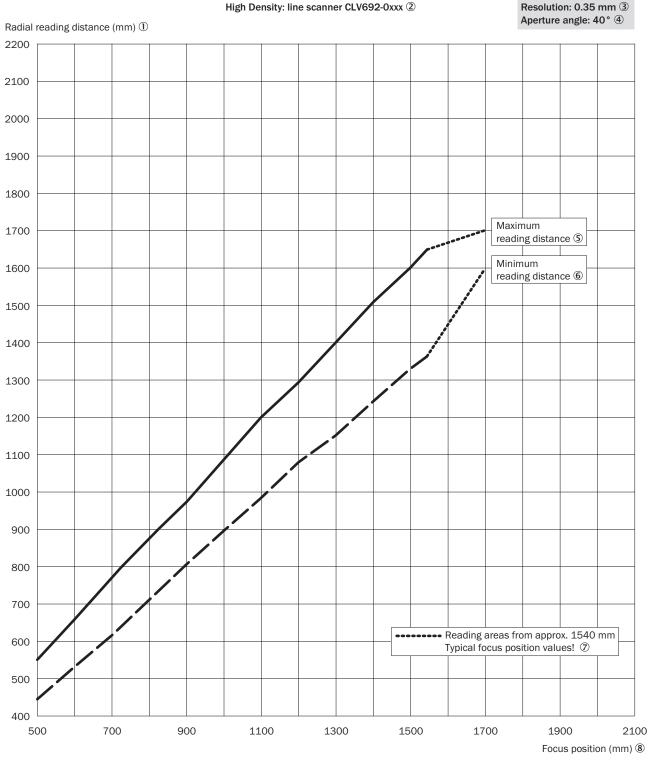
Figure 123: CLV692-0xxx (High Density): min. and max. radial reading distance depending on the focus position at a resolution of 0.35 mm and aperture angle of  $\alpha = 40^{\circ}$
