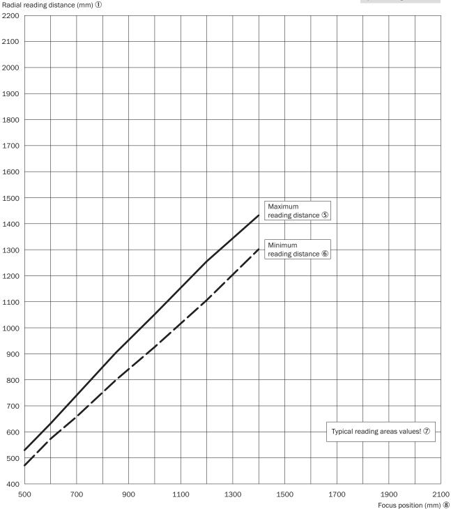
High Density: line scanner with oscillating mirror CLV692-1xxx ②
